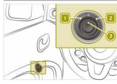
In order to adjust the exterior mirrors electrically, the ignition must be switched on.
