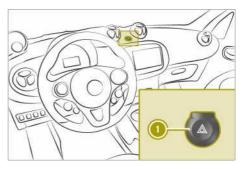
► To switch on the hazard warning lamps manually: press button ①.
