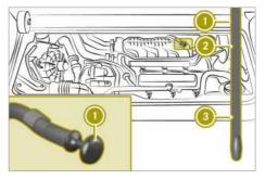
To check the engine oil, the vehicle must be parked on a flat surface.
