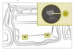
Top tether anchorage (1) is fitted behind each rear seat to the luggage compartment floor.
