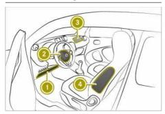
The installation location of an airbag is identified by the AIRBAG symbol.
