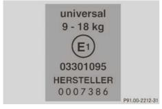
Label for an ECE R44 compliant child restraint system
