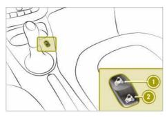
To open or close the folding top, the ignition must be switched on.
