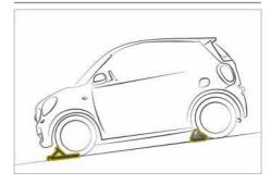
▶ Place wheel chocks or other suitable items in front of the wheels of the front and rear axle.
