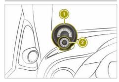
Rev counter ① with dashboard clock ② can be adjusted to the left or right.
