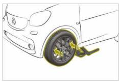
Fit tyres with a specified direction of rotation only according to their direction of rotation. An arrow on the sidewall of the tyre indicates its correct direction of rotation.
