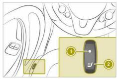
The seat heating only works when the ignition is switched on.
