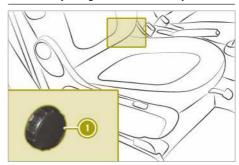
Seat with a handwheel
