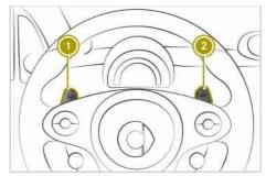
▶ Pull shift paddle ②. The automatic transmission shifts up to the next gear.
