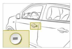
If the vehicle cannot be opened using the remote control key, the vehicle can be opened using the emergency release.
