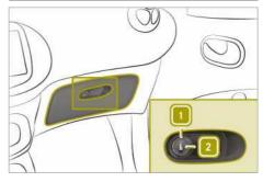
▶ Insert the key into the lock and turn clockwise to position 2 (to lock) or anticlockwise to position 1 (to unlock).
