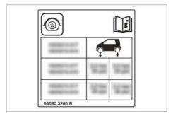
The table with the recommended tyre pressure for various operating conditions can be found on the driver's side door pillar (B-pillar).
