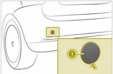
The towing eye can be attached to the front or rear of the vehicle.
