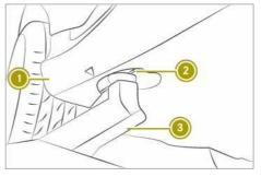
The vehicle may only be raised at the designated jacking points. Points (2) are to the front and back in the immediate vicinity of the wheels. Do not position jack (3) on the edge of sill (1). Otherwise, damage to the vehicle could occur.
