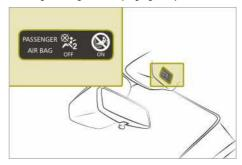
The PASSENGER AIRBAG OFF indicator lamp and PASSENGER AIRBAG ON indicator lamp are part of the front-passenger front airbag deactivation system.
