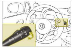
To operate the rear window wiper, the ignition must be switched on.
