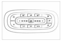
The ignition must be switched on in order to operate the blower. The engine must be running in order to operate all the functions of the automatic climate control system.
