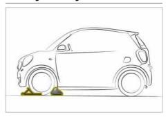
When changing a wheel, place chocks or other suitable items under the front and rear of the wheel that is diagonally opposite the wheel you wish to change.
