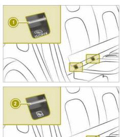
▶ Install the ISOFIX child restraint system on both ISOFIX securing rings (1) or i-Size securing rings (2).
