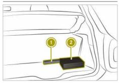
Warning triangle ① is located in the boot behind the seat backrest, secured to the carpet with a Velcro fastener. Return it to this location after use.
