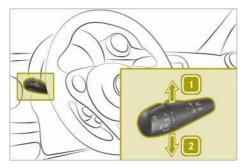
The ignition must be switched on in order to use the turn signals.
