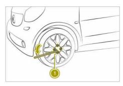
▶ Using wheel wrench (1) loosen the wheel bolts by about one turn. Do not unscrew the wheel bolts completely.
