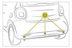
The parking aid uses three sensors (1) in the rear bumper to monitor the area around the
