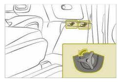
The towing eye and the TIREFIT kit are located in the vehicle tool tray under the glove compartment.
