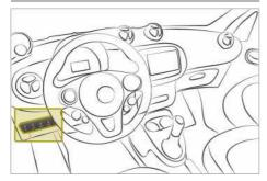
Press the switch. If Lane Keeping Assist is deactivated, the LED on the switch lights up.
