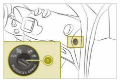
Airbag-off switch ① for manually enabling and disabling the front-passenger front airbag is in the dashboard on the front-passenger side.
