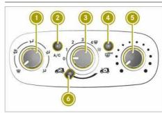
The engine must be running in order to operate the heating and air-conditioning system.
