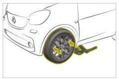
Fit tyres with a specified direction of rotation only according to their direction of rotation. An arrow on the sidewall of the tyre indicates its correct direction of rotation.
