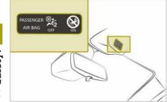
The PASSENGER AIR BAG OFF and PASSENGER AIR BAG ON indicator lamps are part of the front passenger front airbag deactivation system.
